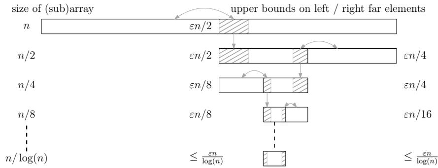
■ **Figure 1** Illustration of the alternating division process using  $\epsilon$ -halvers.
