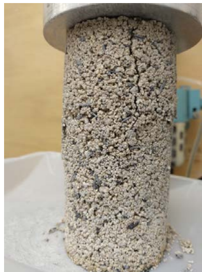
First Crack Appear
