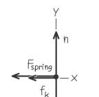
**(c)** Free-body diagram for the glider with kinetic friction
