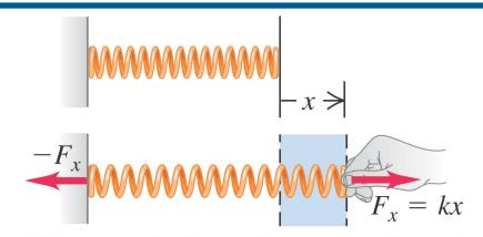
The area under the graph represents the work done on the spring as the spring is stretched from x = 0 to a maximum value X:
