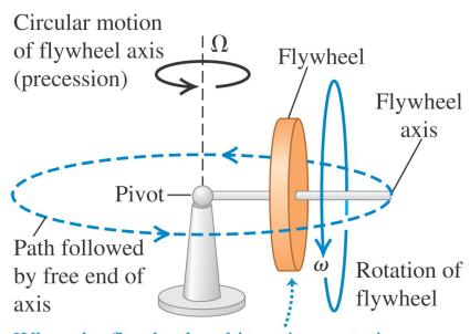
When the flywheel and its axis are stationary, they will fall to the table surface. When the flywheel spins, it and its axis "float" in the air while moving in a circle about the pivot.
