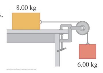
Note: We are able to use conservation of energy because the question did not ask about time (and acceleration). For example, what is the acceleration of the system and how long does it take for the 6kg mass to fall 0.5m?
