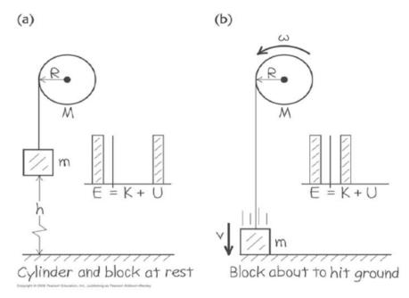
Q. Find the speed of mass m after it has fallen a distance h.
