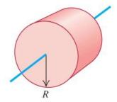
(g) Thin-walled hollow cylinder
