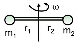
$$K = \frac{1}{2}m_1v_1^2 + \frac{1}{2}m_2v_2^2 = \frac{1}{2}m_1(r_1\omega)^2 + \frac{1}{2}m_2(r_1\omega)^2 = \frac{1}{2}\left[m_1r_1^2 + m_2r_2^2\right]\omega^2$$
