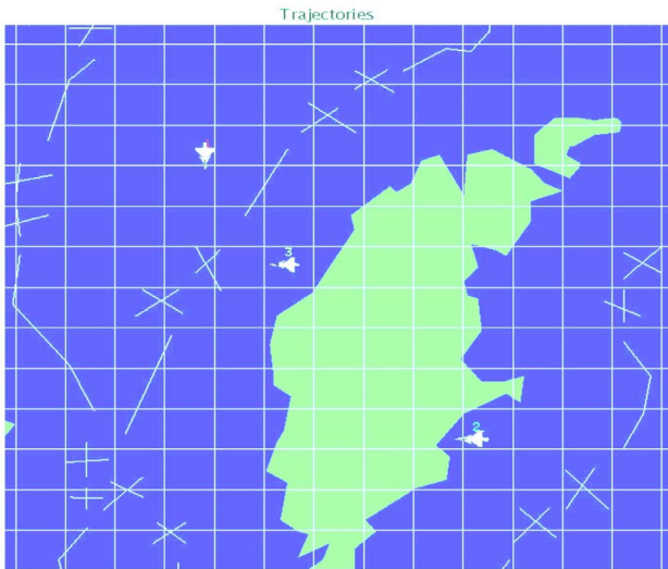
Figure 1: The TACSI simulator display showing one agent controlled aircraft (upper) and two enemy aircraft flying over water (blue/dark) near an island.
