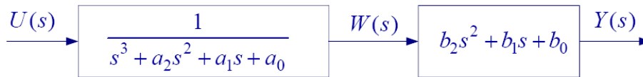
Figure B.4: The transfer function of Eq. (B.9) arranged in cascade form
