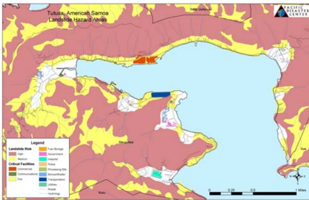
Figure 5: Landslide risk for critical facilities – Pago Pago Harbor area, Tutuila. High-risk areas are marked in red and medium risk in yellow. Derived from USDA, Landslide Mitigation Study , 1990.
