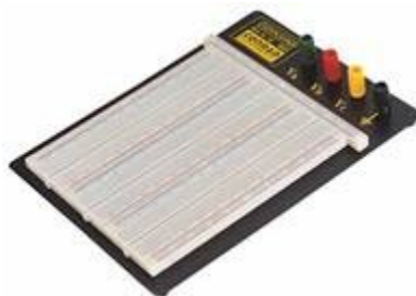
Figure 2: Electronic solderless breadboard, also known as a proto-board.
